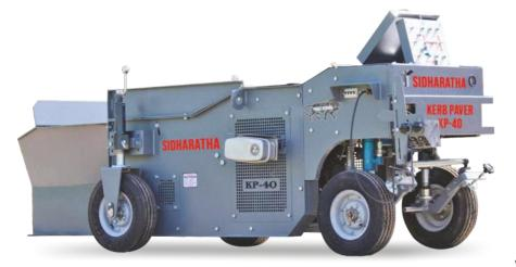
Sidharatha Kerber is a compact machine for laying concrete kerbs of different dimensions, through the extrusion process. An automatic Sensor device provides steering and height control. The use of a zero slump concrete ensures shape true to the mould design. The concrete can be fed into the machine from a Concrete Transit Mixer or a flat bed truck (tractor trolley) be in KP 40.
