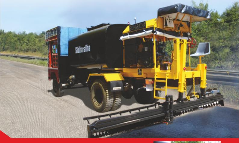
This mobile equipment basically developed for prime coat of bitumen on WMM road surfaces and tack coat on old asphalt paver surfaces . It uniformly sprays hot bitumen or emulsion in exact prescribed quantity Kg/Mt<sup>2</sup> As Per Specifications Laid By IRC OF MoRTH. Capacity Range Available.
